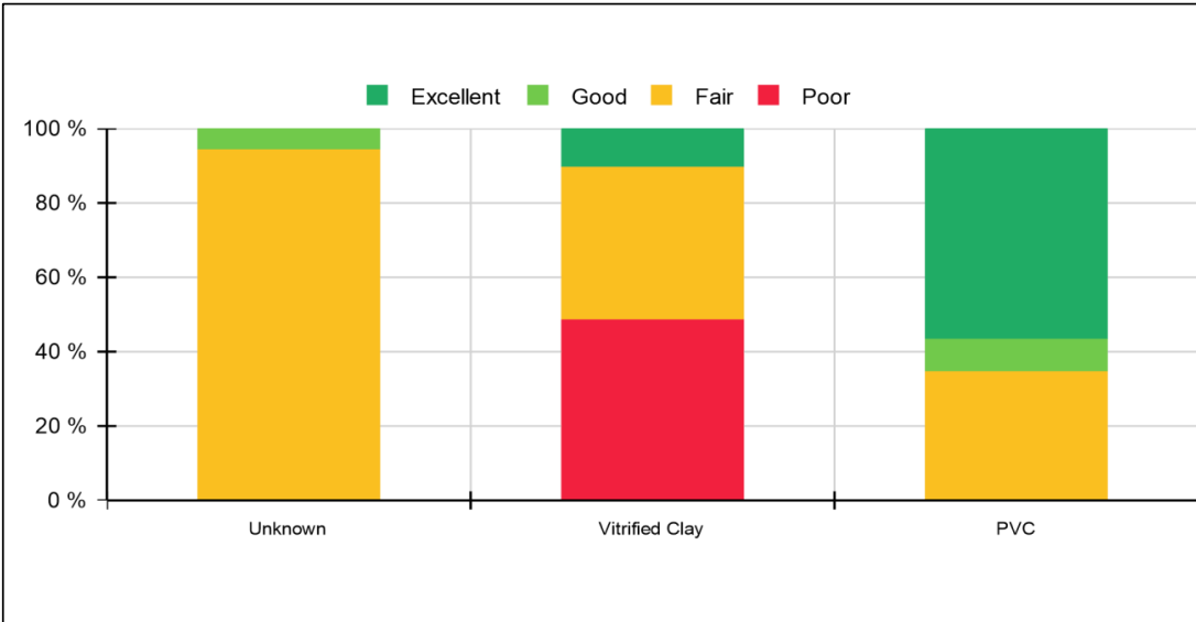
Figure 87: Sewerline Network Condition by Type
