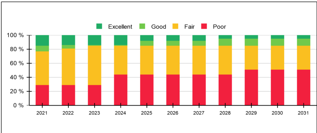
Figure 96: Annual Sewer Manhole Network Condition Status
