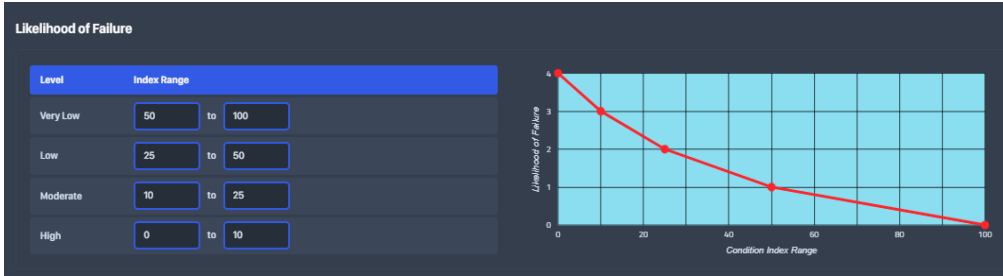
Figure 6: Likelihood of Failure Setting
